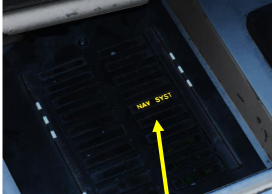
NAV SYST: Navigation System Failure/Malfunction
