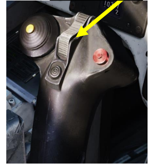
Radar Fix Trigger • T0: Neutral • T1: First trigger detent • TV: Second trigger detent
