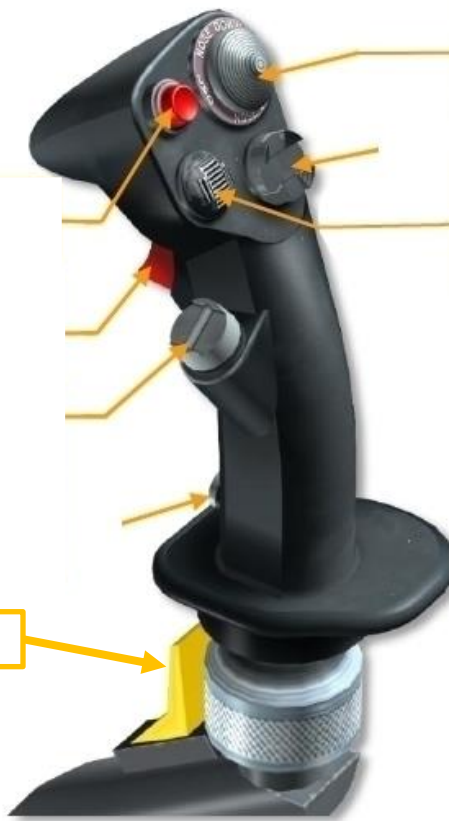
Countermeasures Mode Selector (KB) A: Automatic 0: Off 1: Mode 1 2: Mode 2 3: Mode 3
