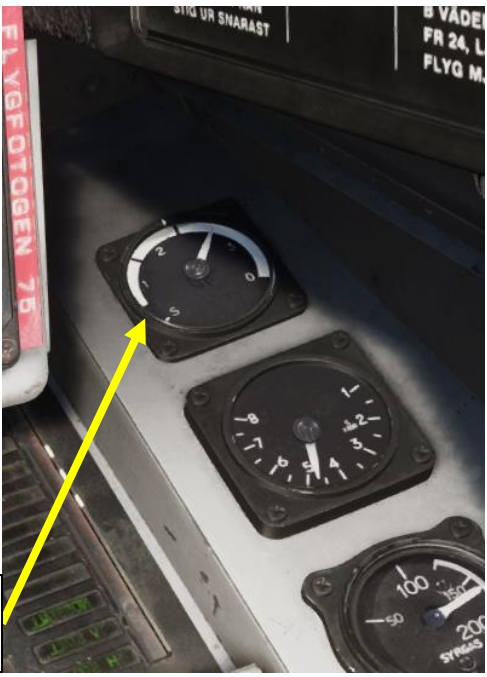
Engine Nozzle Position Indicator (Shown: Afterburner Stage 3)
