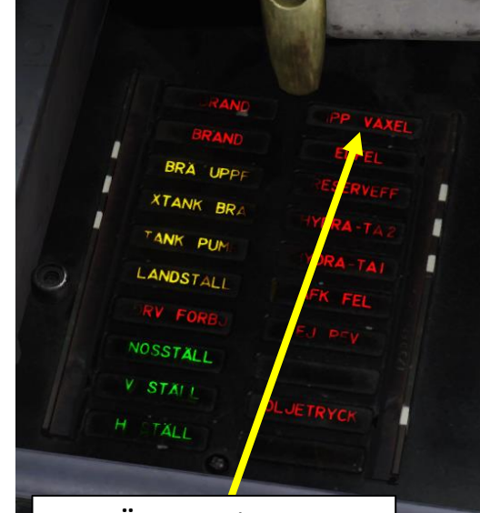
TIPPVÄXEL: Pitch gearing in incorrect mode based on current airspeed
