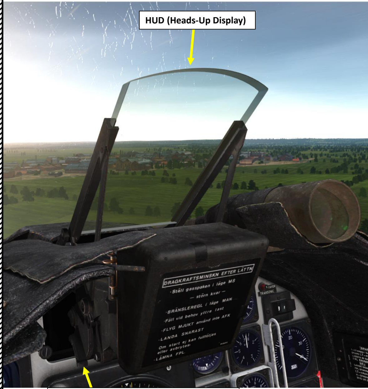
HUD Reflector Glass Position Lever (DOWN)
