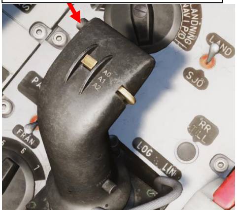
Radar Terrain Avoidance Selector
