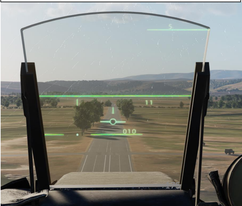
HUD (Heads-Up Display) in LANDN NAV – Prior to Touchdown
