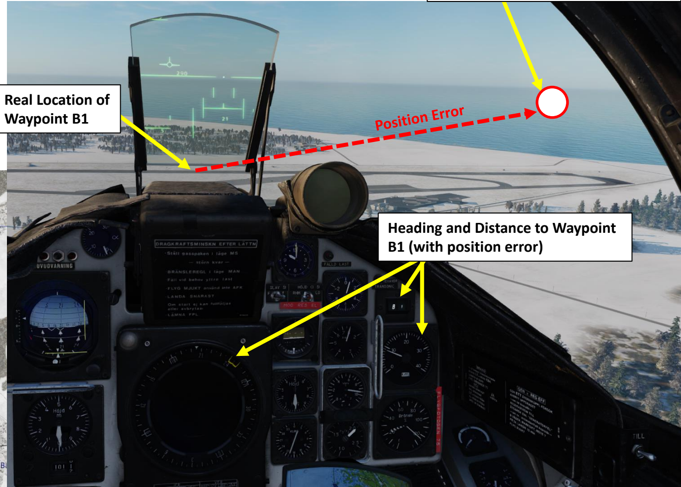
Location of Waypoint B1 perceived by the aircraft (with drift error)
